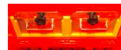
Sowing shaft cover with polyurethane
