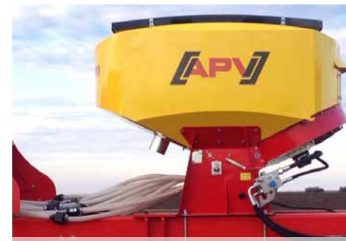
Here, the seed is metered on 32 seeding coulters.
