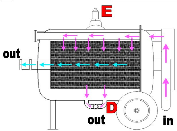
EKOFILTRO ADVANTAGES: doesn't stop the water supply during the backwashing doesn't reduce the water capacity during the backwashing automatic removal of the dirty automatic cleaning of the screen with water flow the bigger filtration surface area in the automatic filters range reduction of water waste
